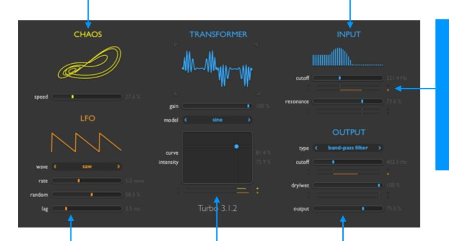
Modulation depth sliders adjust positive or negative (inverse) parameter modulation by the LFO and chaos.
