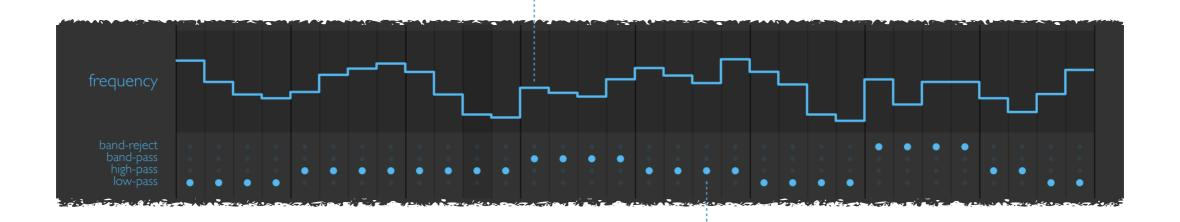
Filter **mode**: click and drag to adjust filter mode for each sequencer step (low-pass, high-pass, band-pass, band-reject), other actions available via <u>shortcuts</u>
