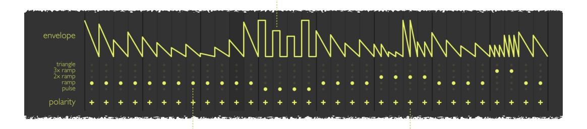
Envelope **shape**: click and drag to adjust envelope shape for each sequencer step (pulse, 1/2/3x ramp, triangle), other actions also available via <u>shortcuts</u>
